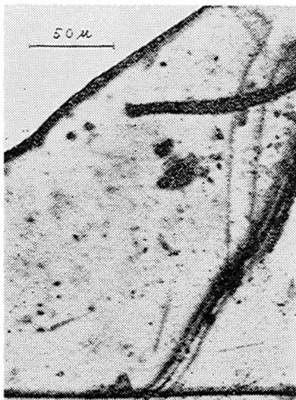
Photograph No. 1—Single crystal which was illuminated by tungsten lamp for 2 hrs.
