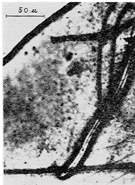
Photograph No. 3—Single crystal which was warmed at 90^\circ\text{C} for 20 mins.
