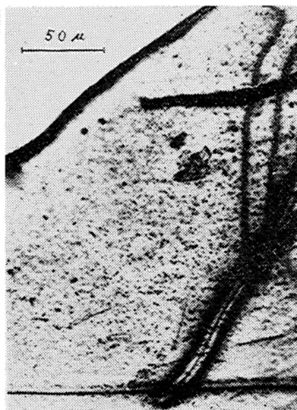
Photograph No. 2—Single crystal which was illuminated by tungsten lamp for 18 hr.
